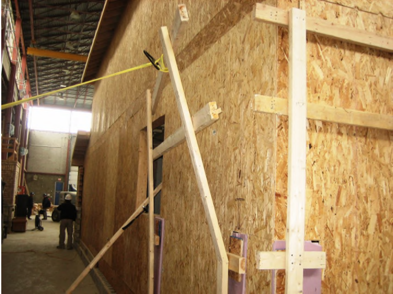
Figure 7: Third and Fourth trials – the post broke at the attachment and the guardrail pulled out from the corners after the post failed. The maximum pull force was over 510 lb.
