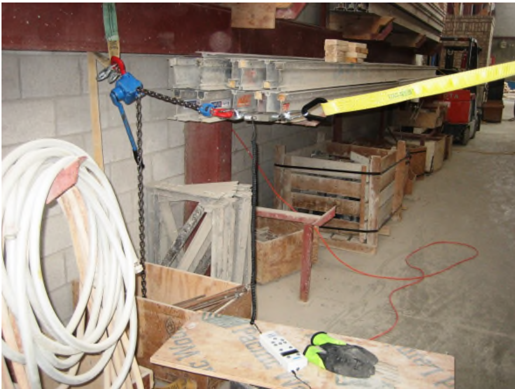
Figure 4: A 5000 lb force cell was used to measure the peak forces.
