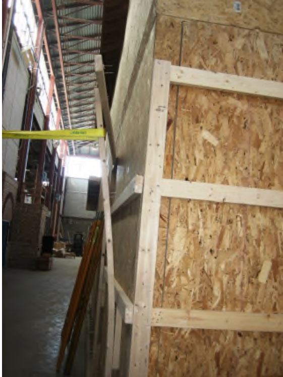
Figure 5: The top rail failed first, follow by the mid-rail.
