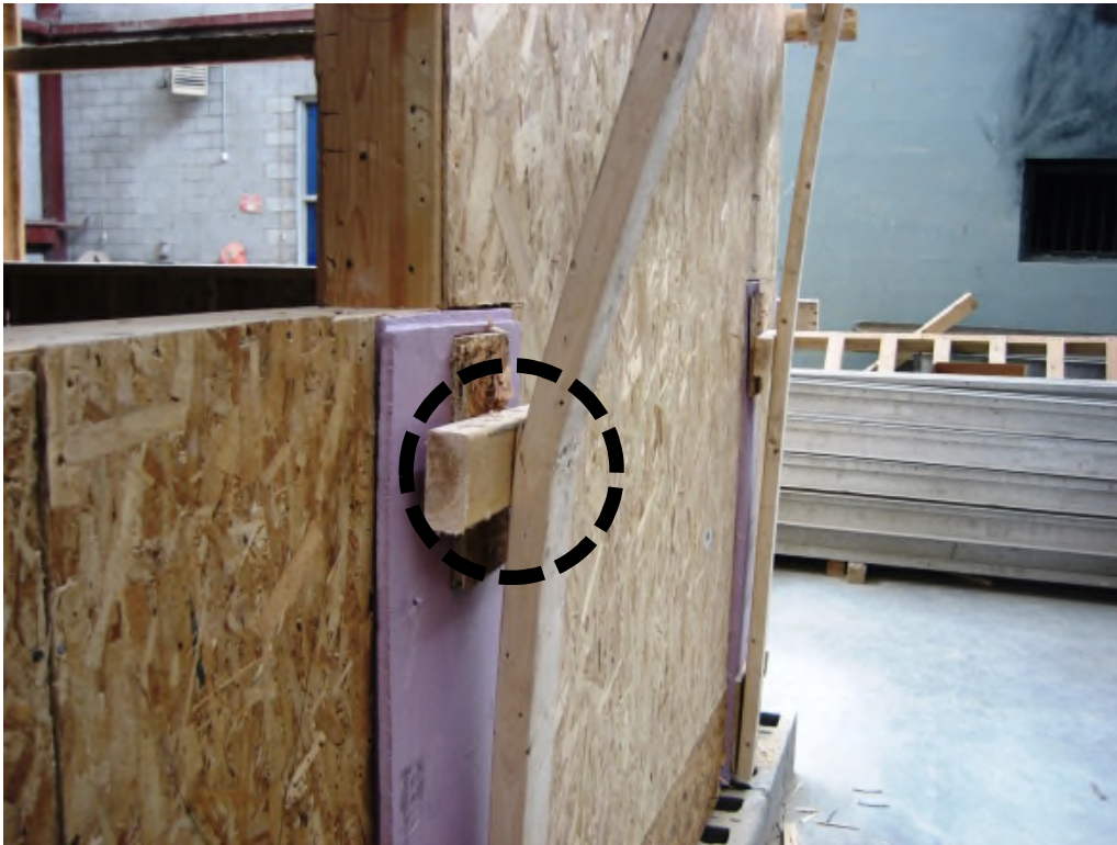
Figure 6: Second trial – the post broke at the attachment. The maximum pull force was 256 lb.
